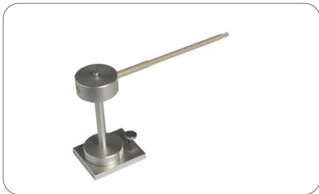
| Figure 7. 8 mm FOV specimen holder
